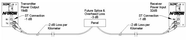
Typical Multimode Fiber Optic Network Cable dB Loss Diagram
