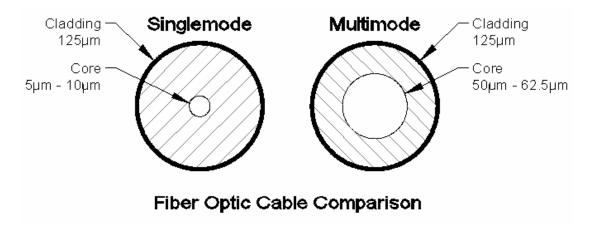
Typical multimode fiber characteristics are: 62.5/125 um, 1310nm, -1 to -2 db/km loss.
