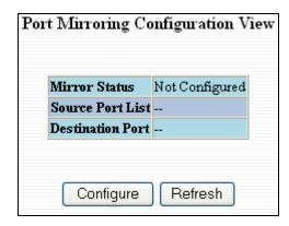
Following the Configure button, you can enable the status of port mirroring and select source ports and the destination port that the source ports will be mirrored to.
