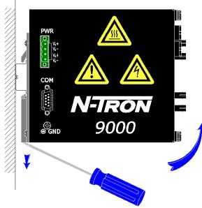
To remove the unit from the 35mm din-rail, place a flat head screwdriver into the release clip at the bottom of the unit, and push down on the clip until it disengages from the bottom of the unit from the din-rail. Lift the bottom of the unit up at an approximate  $45^{\circ}$  upward angle to completely remove the unit.
