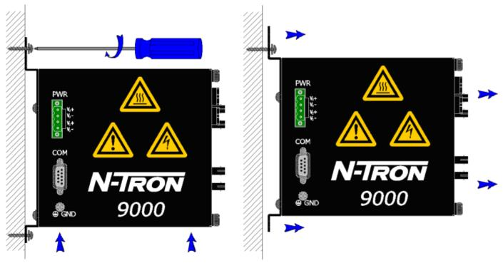
To remove the unit from a wall, remove the bottom two screws that secure it to the wall and slide the unit up until the top two screws will fit through the larger holes on the unit. The switch should then freely come away from the wall.
