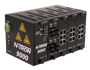
The N-TRON 9000 Series Gigabit Ethernet Capable Industrial Ethernet Switch offers outstanding performance and ease of use. It is ideally suited for connecting Ethernet enabled industrial and or security equipment and is a fully managed switch.
