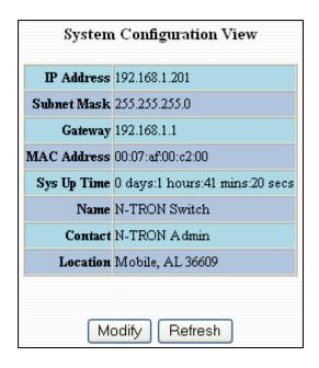
By selecting the modify button you will be able to change the switch's IP Address, Subnet Mask, Default Gateway, Name, Contact information, and the Location of the switch through the web management features. It is recommended to change the TCP/IP information through the Command Line Interface (CLI) initially, but it defaults to the following:
