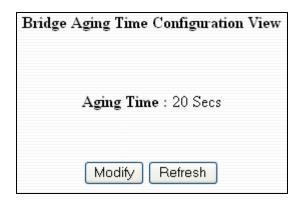
After selecting the Modify button the user will be presented with a page that allows the number to be entered into and updated. The default aging time is 20 seconds.
