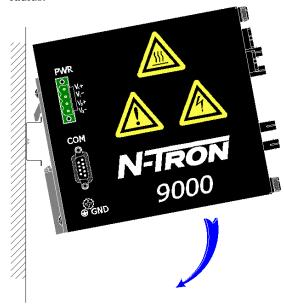
To mount the unit to the 35mm din-rail, place top edge of the bracket on the back of the unit against the din-rail at a  $45^{\circ}$  upward angle. Lower the bottom of the unit until it snaps into place.
