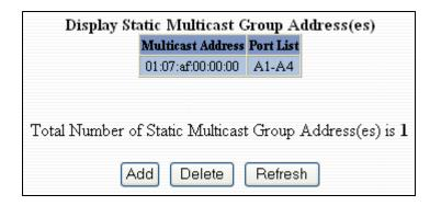
Following the Delete button on the page above, the administrator will be presented with a list of Multicast Group Addresses that are configured on the switch. Using the pull down menu the administrator should select the desired port to be removed. Then click on the Delete button at the bottom of the page.
