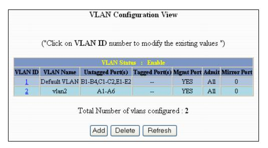
To delete or remove VLANs that are no longer wanted simply click on the Delete button on the main Port Based VLAN page. That button will load the page where the user can enter the VLAN ID that he or she wishes to delete.
