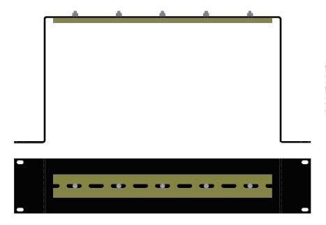
Most N-Tron<sup>TM</sup> products are designed to be mounted on industry standard 35mm DIN-Rail. However, DIN-Rail mounting may not be suitable for all applications. Our Rack Mount Assembly (P/N: 900-RM) may be used to mount the 9000 Series to standard 19" racks as an option.
