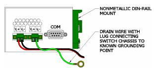
Both V- legs of the power input connector are connected to chassis internally on the PCB. Connecting a drain wire to earth ground from one of the V- terminal plugs as shown here will ground the switch and the chassis. The power leads from the power source should be limited to 3 meters or less in length.
