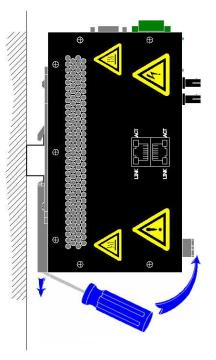
To mount the unit to the 35mm din-rail, place top edge of the bracket on the back of the unit against the din-rail at an upward angle. Lower the bottom of the unit until it snaps into place.
