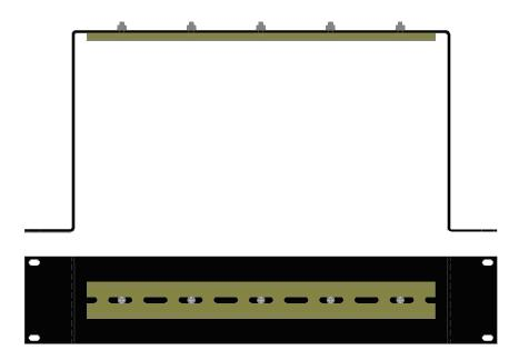
Most N-Tron<sup>TM</sup> products are designed to be mounted on industry standard 35mm DIN-Rail. However, DIN-Rail mounting may not be suitable for all applications. Our Rack Mount Assembly (P/N: 900-RM) may be used to mount the 7014 Series to standard 19" racks as an option.
