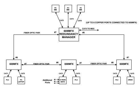
(UP TO 6 COPPER PORTS CONNECTED TO EACH 608MFX)
