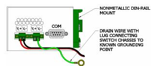
Both V- legs of the power input connector are connected to chassis internally on the PCB. Connecting a drain wire to earth ground from one of the V- terminal plugs as shown here will ground the switch and the chassis. The power leads from the power source should be limited to 3 meters or less in length.
