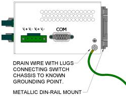
The use of shielded cables between devices is not required for most N-Tron devices (please consult the user manuals for specific details). If the use of shielded cables is required, it is generally recommended to only connect the shield at one end to prevent ground loops and interfere with low level signals (i.e. thermocouples, RTD, etc.). Cat5e cables manufactured to EIA-568A or 568B specifications are required for use with N-Tron Switches.
