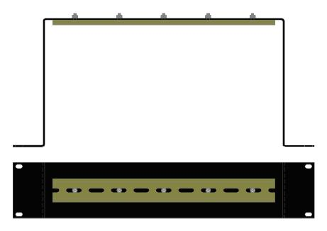
Most N-Tron<sup>TM</sup> products are designed to be mounted on industry standard 35mm DIN rail. However, DIN rail mounting may not be suitable for all applications. Our Rack Mount Assembly (P/N: 900-RM) may be used to mount the 102RAS to standard 19" racks as an option.
