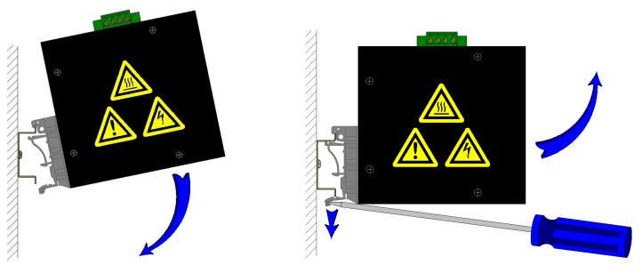
To mount the unit to the 35mm DIN rail, place top edge of the brackets on the back of the unit against the DIN rail at a  $45^{\circ}$  upward angle. Lower the bottom of the unit until it snaps into place on each bracket.
