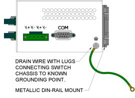
The use of shielded cables between devices is not required for most N-Tron devices (please consult the user manuals for specific details). If the use of shielded cables is required, it is generally recommended to only connect the shield at one end to prevent ground loops and interfere with low level signals (i.e. thermocouples, RTD, etc.). Cat5e cables manufactured to EIA-568A or 568B specifications are required for use with N-Tron Switches.
