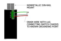
The use of shielded cables between devices is not required for most N-Tron devices (please consult the user manuals for specific details). If the use of shielded cables is required, it is generally recommended to only connect the shield at one end to prevent ground loops and interfere with low level signals (i.e. thermocouples, RTD, etc.). Cat5e cables manufactured to EIA-568A or 568B specifications are required for use with N-Tron Switches.
