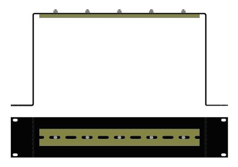
Most N-Tron<sup>TM</sup> products are designed to be mounted on industry standard 35mm DIN rail. However, DIN rail mounting may not be suitable for all applications. Our Rack Mount Assembly (P/N: 900-RM) may be used to mount the 100 Series enclosures to standard 19" racks as an option.
