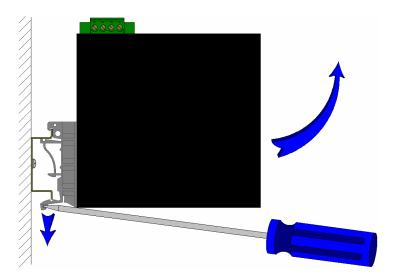
To remove the unit from the 35mm industrial DIN rail, place a flat head screwdriver into the release clip found at the bottom of the unit, and apply downward force on the clip until it disengages from the bottom of the unit from the DIN rail. Rotate the bottom of the unit towards you and up at an approximate 15° upward angle to completely remove the unit.
