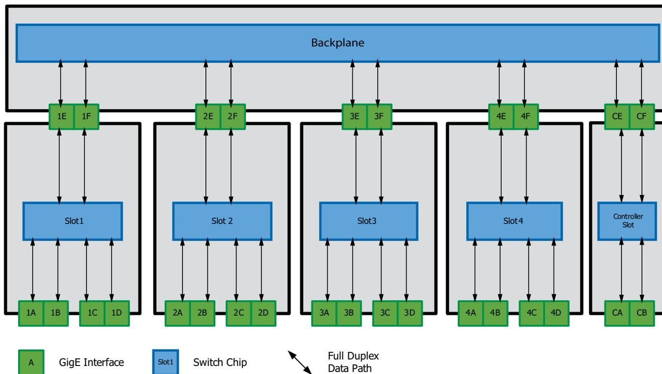
Figure 16: SmartNA System: Port Nomenclature & Connections
