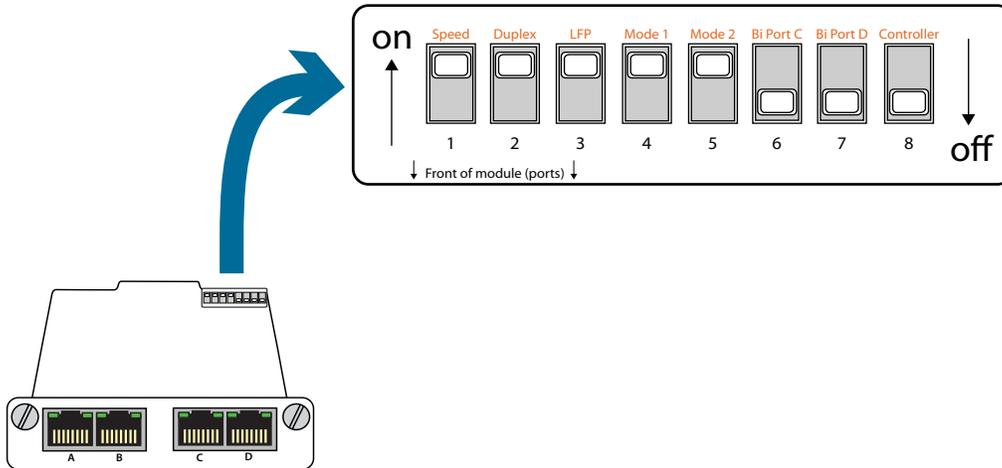
**Figure 31:** Location of DIP switches on the V-Line TAP
