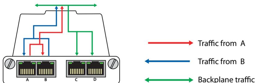
**Figure 22:** Backplane Aggregating mode
