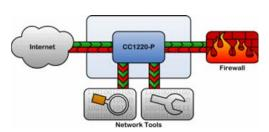
In COMBI mode bi-directional live network traffic is combined onto each monitor port, in this way two network tools can be given access to the traffic. This type of deployment is recommended for edge links where traffic levels are lower.
