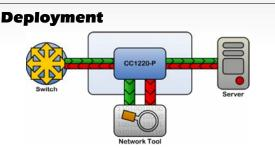
In BREAKOUT mode bi-directional live network traffic is broken-out onto separate monitor ports, giving a single network tool full access to the traffic. This type of deployment is recommended when 100% guaranteed traffic capture is required.
