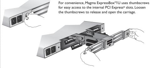
Adjustable card retainers should be used to hold the PCI Express cards securely in place. Use the thumbscrews to loose and rotate the card retainers to the appropriate position for securing the card.
