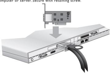
Connect one end of the PCI Express cable to the Magma PCIe Host card installed in the host computer. Connect the power cords and other end of PCIe cable at the rear of the enclosure.
