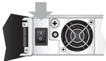
NOTE: There are two power supply modules included in ExpressBox<sup>4</sup>. Ensure that the ON/OFF switch is in the ON position.
