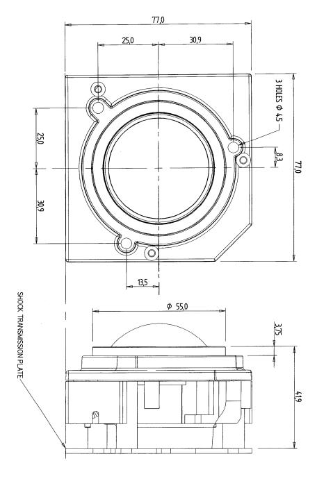
Note: Shock transmission plate is optional Bezel height is dependent on choice of bezel type. Contact us for more details.
