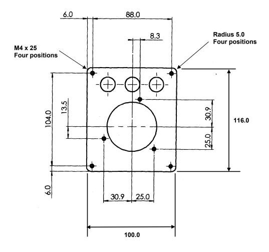
Panel thickness is 2.0mm. Grain direction is north-south.
