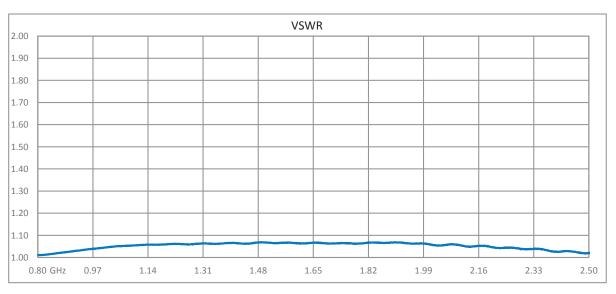
Click the following link (or enter part number in "SEARCH" on website) to obtain additional part information including price, inventory and certifications: TNC F/F Coaxial RF Surge Protector, 800MHz - 2.5GHz, 300W, IP67, 15 V Max., 500uJ, 20kA, Hybrid, Bracket Down, Hole Mount DGXZ+15TFTF-A
